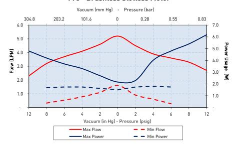
The above graph represents an example of performance for the pumps series handling air at 800 feet (244m) above sea level at 75°F (24°C). Performance will vary depending on barometric pressure and media temperature. Curves are representative of standard pump configurations. Pump configurations could be customized for higher or lower flows, depending on specific customer requirements.
