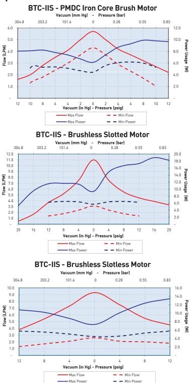
The above graph represents an example of performance for the pumps series handling air at 800 feet (244m) above sea level at 75°F (24°C). Performance will vary depending on barometric pressure and media temperature. Curves are representative of standard pump configurations. Pump configurations could be customized for higher or lower flows, depending on specific customer requirements.
