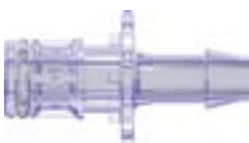
RQCM655 (-9024 -001) RQCM655 (-6005 -001) Male Open Flow, 600 Series Barb, Platinum-Cured Silicone O-Ring, 1/4" (6.4 mm) Tubing ID
