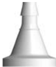
SFMN655 (-6005 -J1A) Sanitary Fitting, Mini Flange 3/4" to 600 Series Barb, 1/4" (6.4 mm) Tubing ID
