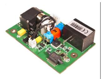
Sidestream capnography module with Integrated T2-05 LI and X-Valve
