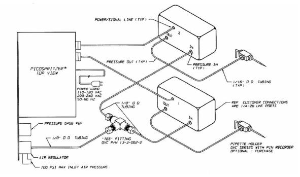
Note: Single channel models have only one valve box and the "tee" fitting is omitted.
