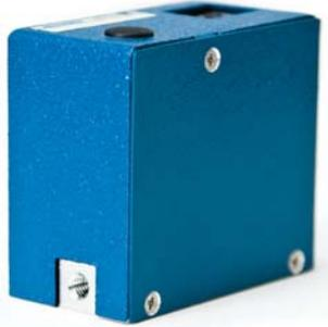
The VSO-GC, Electronic Pressure Control (EPC) Unit, converts a variable electrical control signal into a variable pneumatic output. By providing integral closed loop control, it replaces manual regulators, costly multiple function control valves, and needle valves. This product uses Parker Hannifin's patented VSO® proportional valve and offers application-specific integrated pneumatic pressure control for Gas Chromatography (GC) applications.
